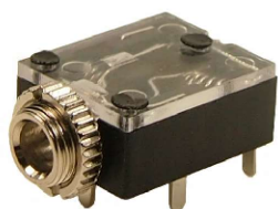
JYS-35 stereo switched 3.5mm Jack Socket. Right angle PCB mounting. Supplied with ring nut.
