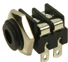
S6/BB mono switched 3.5mm Jack Socket. Panel mounting with solder tags. Also available with Special 'C' Contact to suit Far Eastern plugs.
