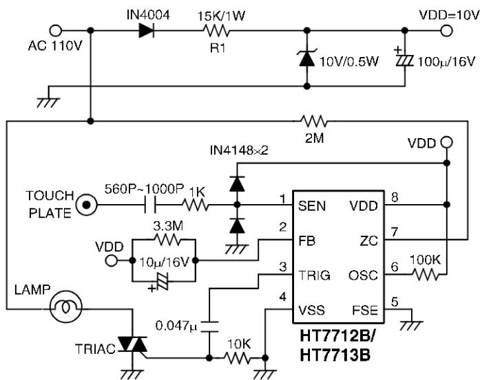
Note: 1. In 220V AC line power, the R1=33K/1W
