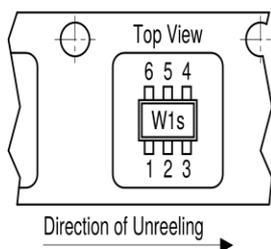
Marking on SOT-363 package (for example W1s) corresponds to pin 1 of device
