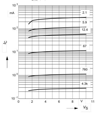
**Collector current**  $I_C = f(R_{ext.})$  of stabilized NPN Transistor
