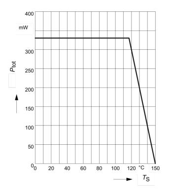
Note that up to  $T_{\rm S}$ =115°C it is not possible to exceed  $P_{\rm tot}$  respecting the maximum ratings of  $V_{\rm S}$  and  $I_{\rm Contr.}$  The collector or drain current (respectively) of the stabilized RF transistor does not affect BCR 400 directly, as it provides just the base current.
