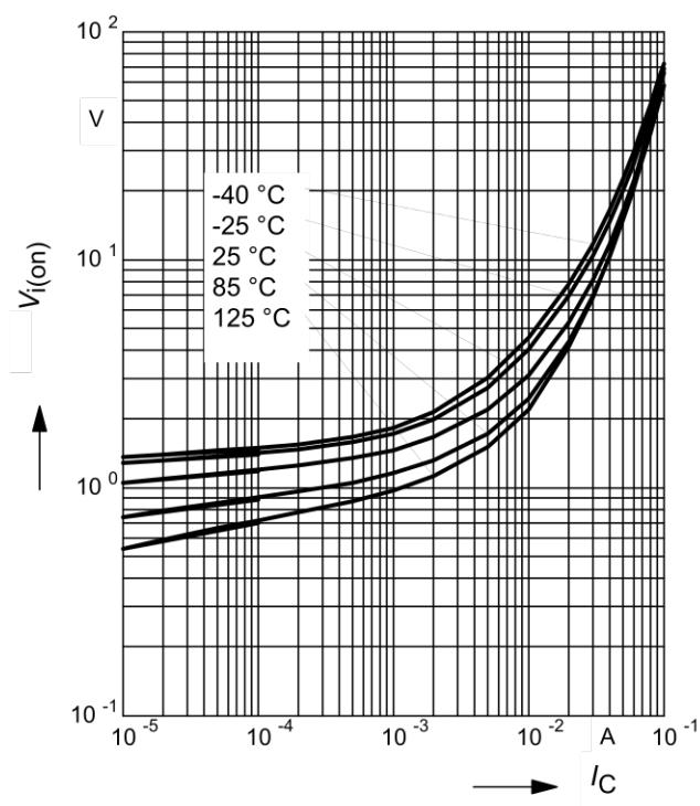
**Collector-Emitter Saturation Voltage**
