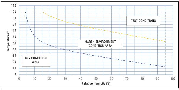
The dry condition area is defined as the range of temperature and relative humidity to validate the life time and  $V_{rms}/I_{rms}$  graphs. The separation line between harsh environment conditions and test conditions area is calculated for a life time of one year at operating voltage.
