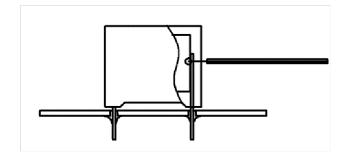
Temperature monitored inside the capacitor.
