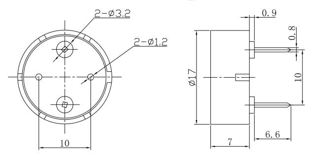
HOUSING METERIAL: NORYL WAVE SOLDER AND WASH NOT ALLOWED.
