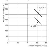
Note: The maximum coil voltage refers to the maximum value in a varying range
