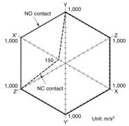
Sample: G2RL-24 12 VDC Number of Relays: 5 pcs Test conditions: Shock is applied in ±X, ±Y, and ±Z directions three times each with without energizing the Relays to check the number of
