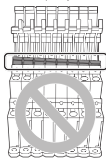
Incorrect installation Some terminals not inserted completely.
