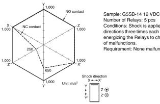
Number of Relays: 5 pcs Conditions: Shock is applied in ±X, ±Y, ±Z directions three times each with and without energizing the Relays to check the number of malfunctions. Requirement: None malfunction 100 m/s<sup>2</sup>
