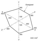
Sample: G6B-1114P-US Number of Relays: 12 pcs Test Conditions: Shock is applied in  $\pm X$ ,  $\pm Y$ , and  $\pm Z$  directions three times each with without energizing the Relays to check the number of malfunctions. Requirement: None malfuction 100 m/s²
