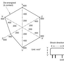
Sample: G6C-2114P-US DC24V Number of Relays: 6 pcs Test conditions: Shock is applied in ±X, ±Y, and ±Z directions three times each with without energizing the Relays to check the number of malfunctions. Requirement: 100 m/s²
