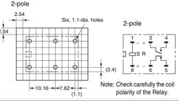
Fully Sealed Model Single Latching Models G6CU-□114P-US
