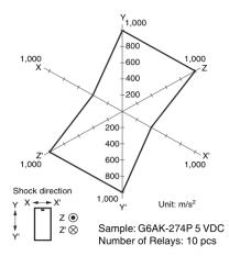
Test Conditions: Shock is applied in  $\pm X$ ,  $\pm Y$ , and  $\pm Z$  directions three times each with and without energizing the Relays to check the number of contact malfunctions.
