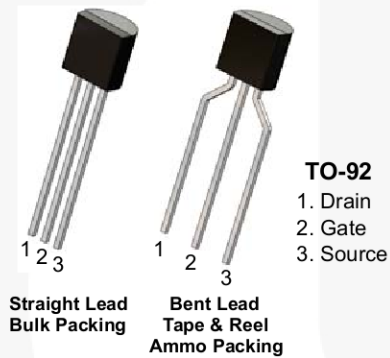
Figure 1. J175 / J176 Device Package
