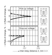
5-(2). Influence of adjacent mounting (2 Form C) Pick-up voltage (1) (2) (3) change, ►Rate of 111 ►Rate of change, % Drop-out voltage 10 5 197 Inter-relay distance ℓ, mm inch
