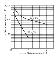
3. Contact reliability for AC loads Tested sample: DS2E-S-DC24V 10 pcs. Operating speed: 20 cpm.
