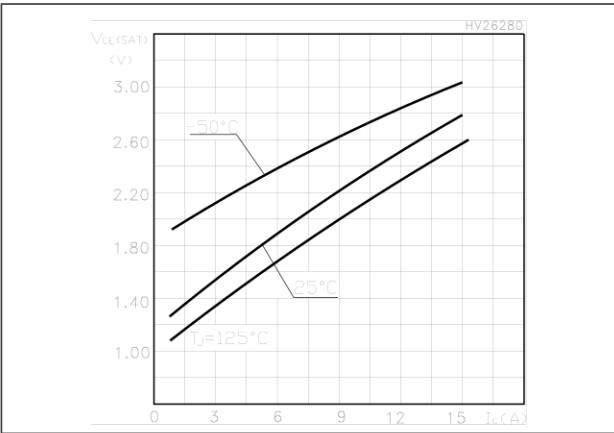
Figure 6. Collector-emitter on voltage vs collector current
