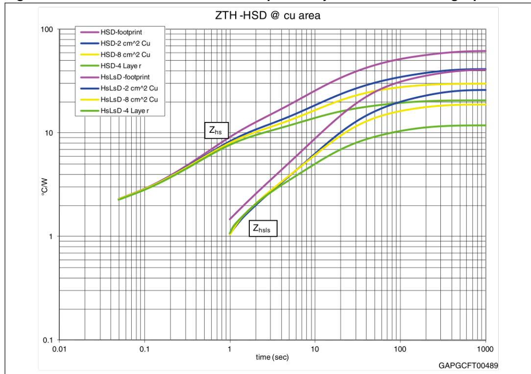
Figure 15. PowerSSO-36 HSD thermal impedance junction ambient single pulse
