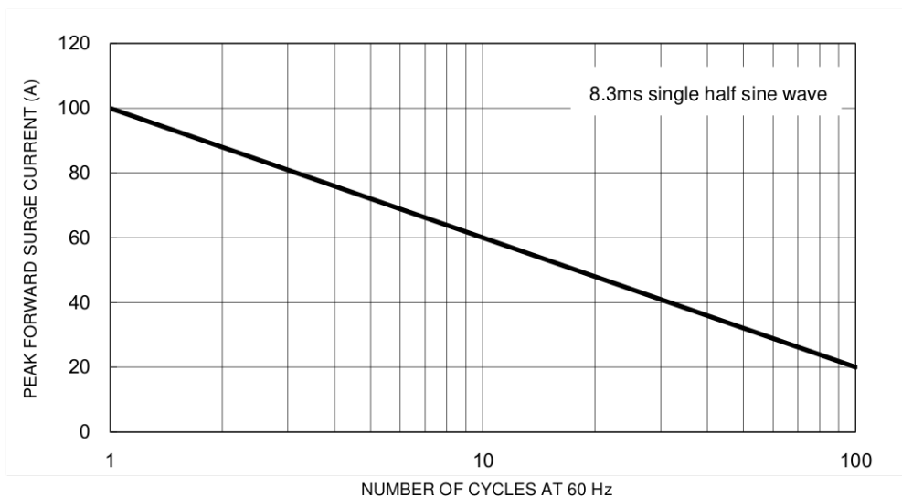
Fig.5 Maximum Non-Repetitive Forward Surge Current
