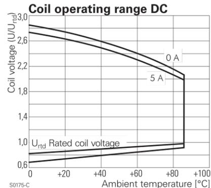
All figures are given for coil without pre-energization, at ambient temperature +23°C. Other coil voltages on request.
