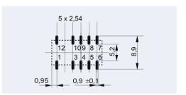
Note: Hole for pin 6 and 7 only for latching with 2 coils. Basic grid 2.54 mm
