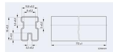
Tube for THT version 50 relays per tube 2'000 relays per box
