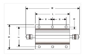
6 x Mounting Hole HSC200 - 5.3mm HSC250 - 5.3mm HSC300 - 6.5mm
