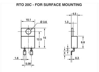
Only for RTO 20 version C = during surface mount soldering temperature profile must not cause the metal tab of this device to exceed 220  $^{\circ}\text{C}.$
