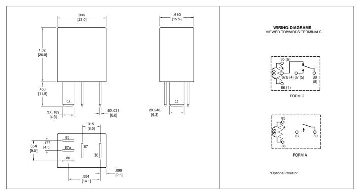
Dimensions in inches with metric equivalents in parentheses. Tolerance:  $\pm$  .010"
